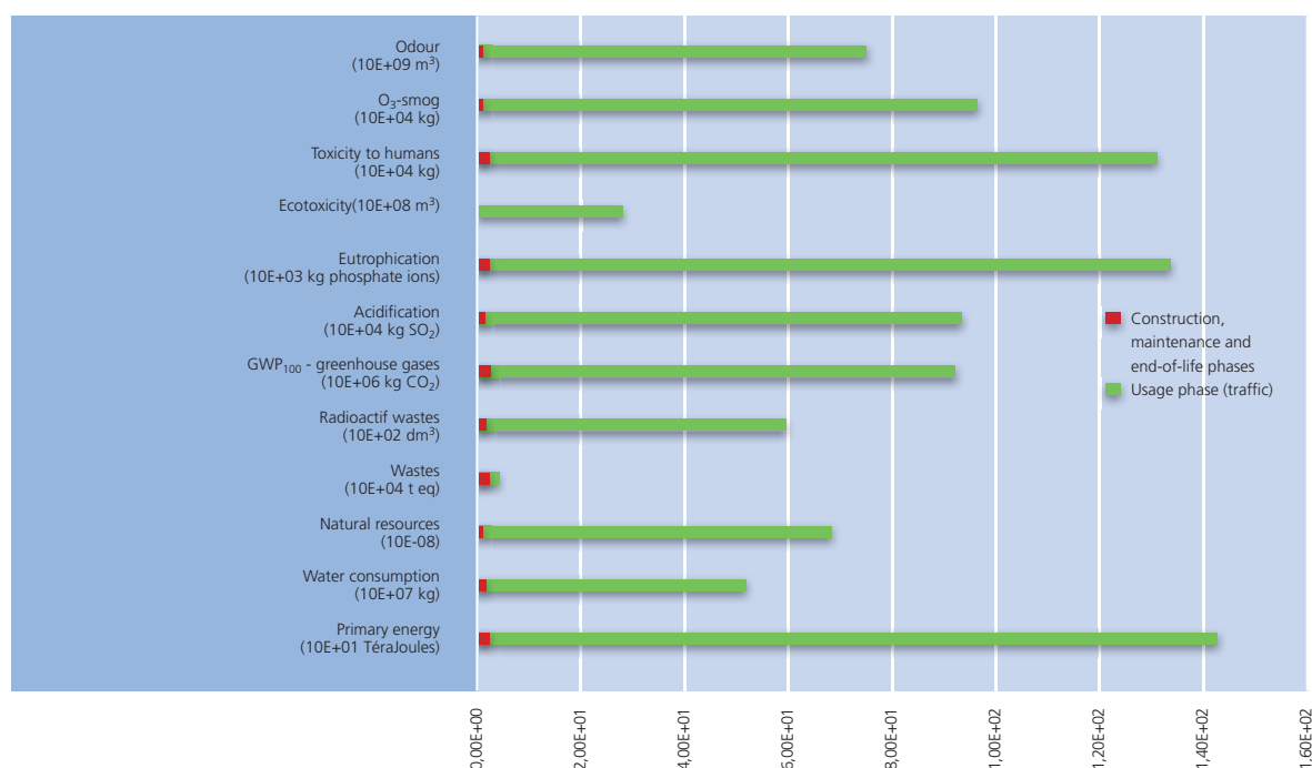
Figure 2 : Lifetime impact of a jointed plain concrete road including traffic for various environmental indicators
